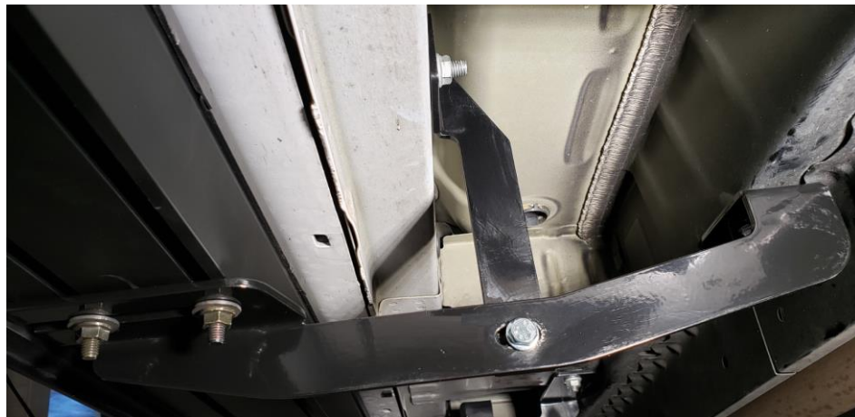
Image shows pass middle bracket installed
