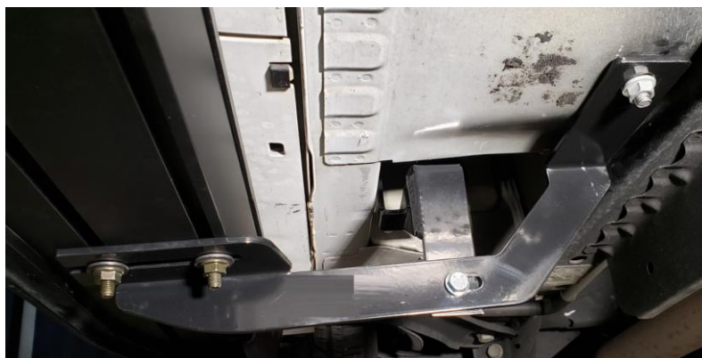
Image shows pass rear bracket installed
