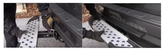
**Step 3:** Install special bolt, using a 22mm socket or wrench tighten bolt until hitch does not move. Install safety pin, you have completed the installation.
