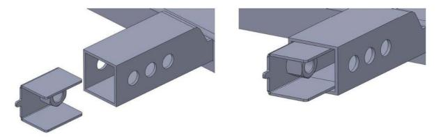
**Step 2:** Slide hitch step into 2-inch receiver. Make sure to choose one of three positions.
