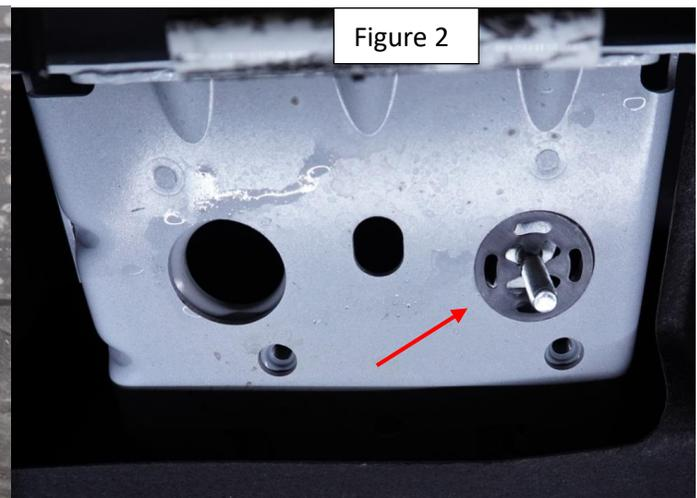
**Step 2:** Install front bracket using supplied M10 bolt and HTC 328 as shown on Figure 3 Note: Some vehicles may require chasing the threads to remove extra paint or dirt before installing 10mm bolt. Do not fully tighten.
