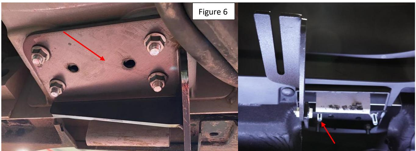
**Step 6:** Proceed to last page of this manual for running board install instructions and torque values Max torque is 7 ft lbs. Do not overtighten as this may damage the running boards.
