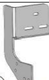
3 2013850R0 DRIVER SIDE REAR/ PASSENGER SIDE FRONT-MIDDLE BRACKET 3 x QTY
